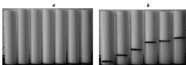
Figure 1. Photographs of emulsions prepared with AG (a) and XG (b) after preparation for 12 h at room temperature: (a) concentration of AG in the sequence 0, 0.023, 0.039, 0.060, 0.081, 0.11, and 0.14% from left to right; (b) concentration of XG in the sequence 0.011, 0.019, 0.040, 0.069, 0.10, and 0.15% from left to right.
